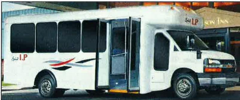
23 Foot Low Floor Cutaway Alternative Fuel Bus
